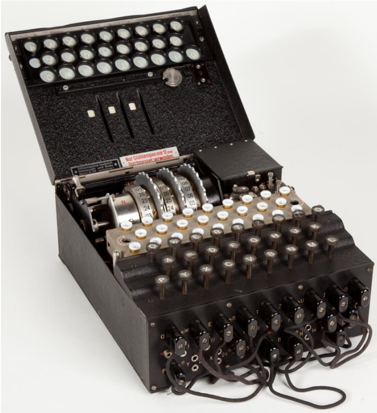
The initial Enigma Machine. Public domain.
